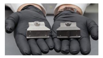
A custom mounting bracket 3D printed on the Desktop Metal Production System P-1 in under two hours. The as-printed part, above left, was then blasted with alumina grit for the final surface finish, above right.
